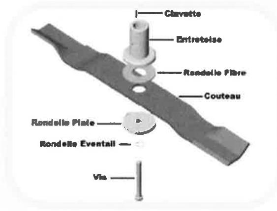
You must regularly check the condition of the blade and of the fibre grommets. You may proceed with their sharpening if necessary.
